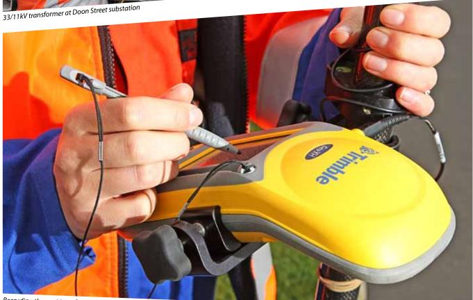
Recording the position of underground cables
