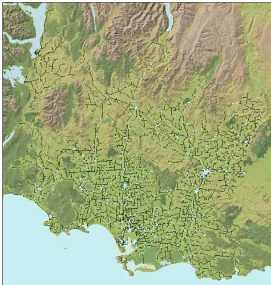
Figure 22 Low Voltage Poles with less than 10 years remaining life
