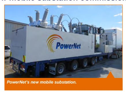
Southland's first mobile substation was commissioned in March after nearly three years in planning and construction. The 15.66m long and 2.5m wide trailer mounted substation comprises a 5MVA transformer, 66kV and 22kV circuit breakers, control room and other auxiliaries.
