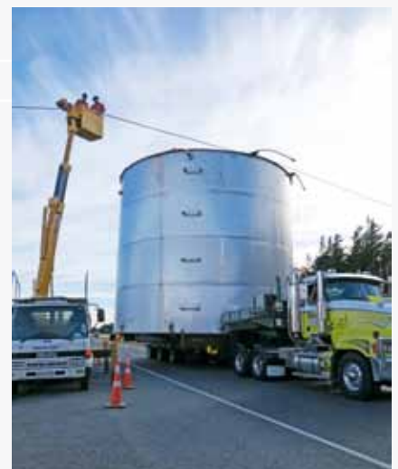
The nitric acid tank passing under TPC electricity lines at Awarua
