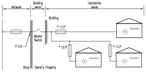
For multiple Installations, PowerNet permits a voltage drop up to 4% between the Point of Supply and the Metering Point.
