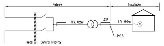
In cases 5.4.2, 5.4.3 and 5.4.4 there may be no LV fuse, as described in section 13.3.2. In these cases, the HV fuse will be classed as the ICP fuse.
