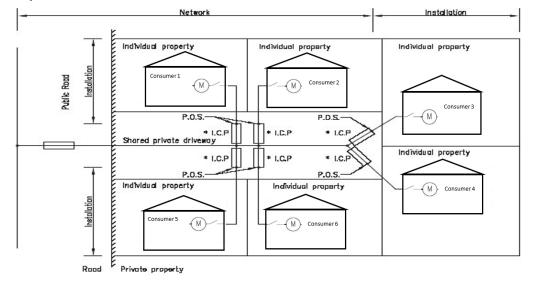
• For 5.3.3 and 5.3.4 these fuses are provided by PowerNet and must be installed in such a manner that access is available to PowerNet authorised staff at all times. This is the ICP for the Installation.
